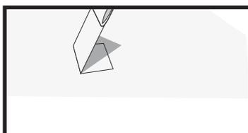
Using a TESA® 7476 adhesive tape, or similar, apply it to a surface of 2.5 cm x 5 cm (1 in. x 2 in.) plus some overhang material for easier removal. Fold and promptly tear it off perpendicularly to the substrate surface. No traces should remain on the ripped-off adhesive tape. Repeat this process in several places.
